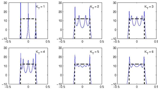
Fig. 4. Effect of increasing  $K_T$ , the number of observations along time direction on the LF time correlation spectrum. The solid lines plot the spectra of LF time correlation sequence whereas the dashed lines plot the rectangular (heuristic) time correlation spectrum for reference. The vertical axis displays the spectrum magnitude in dB while the horizontal axis shows the angular frequency ( $-\pi$  to  $\pi$ ). Note that we show only the central portion of the spectra.
