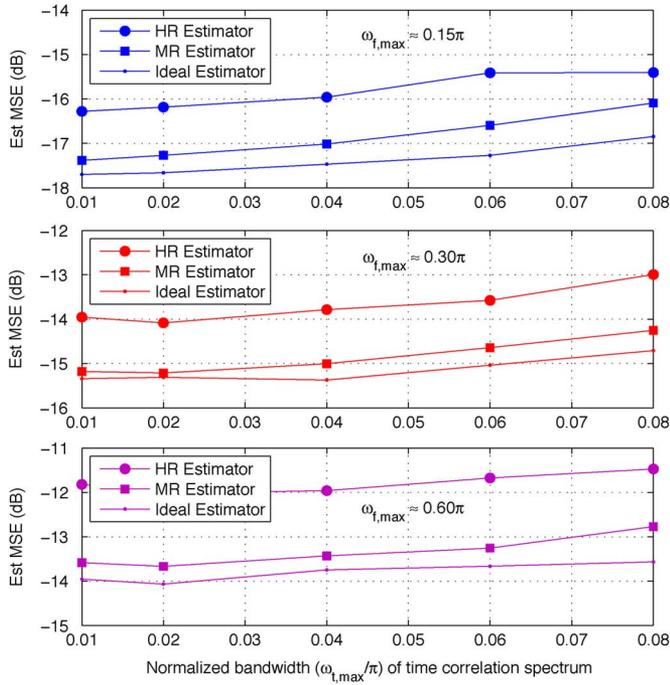
Fig. 2. Worst case channel estimation MSE (at  $\sigma_\eta^2 = 10^{-1}$ ) of the heuristic and proposed estimator. Please refer to the caption of Fig. 1 for further details. Gains of around 1 dB are achieved by the MR estimator.
