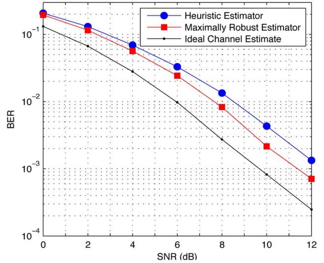
(a) QPSK, Veh-A PDP, Bandpass DS, velocity 120 kmph
